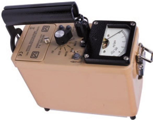
FIG. 7.3. An ion chamber survey meter (Courtesy of Ludlum Instruments, Inc. Sweetwater, TX).
