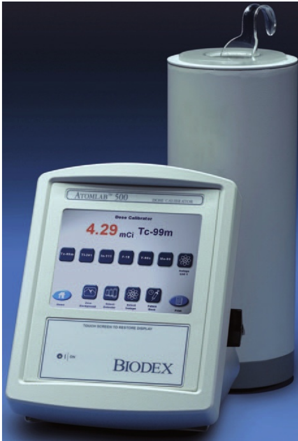
FIG. 7.5. A typical dose calibrator (Courtesy of Biodesx Medical Systems, Inc, Shirley, NY).
