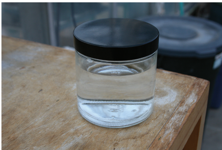
Figure 6.8 Jar test to determine pesticide compatibility.
