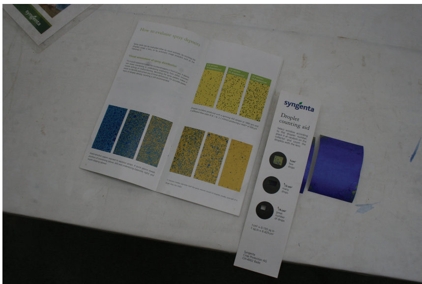
Figure 6.4 Water-sensitive paper with examples of spray droplet patterns.
