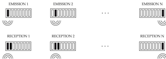
Figure 2. Firing sequences of the elements in 2R-SAFT
