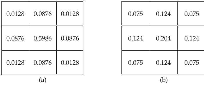
Figure 17. The 3x3 kernel with (a) \sigma = 0.5 , (b) \sigma = 1 .
