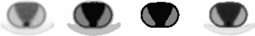
FIGURE 5. Illustration of the segmentation process of a heart/chest phantom transmission images showing from left to right: the original transmission image, FCM segmented image using 5 clusters, merging process to a three-clustered image (the bed is removed here), and the final attenuation map after applying a Gaussian filter and weighted averaging (the low-noise image of the bed acquired and processed off-line is added here).
