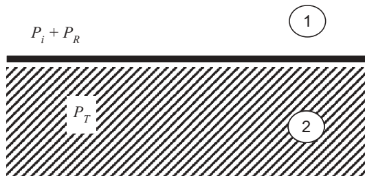
Figure 6.6. The pressure at upper medium (from which the wave has arrived) is comprised of the pressures generated by the incident and reflected waves. At the boundary between two mediums the pressure on both sides should be equal.
