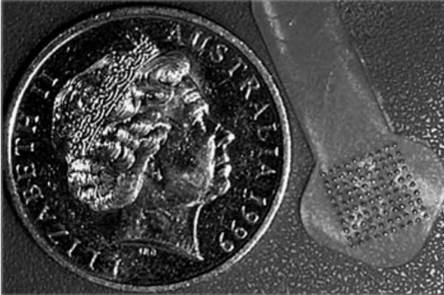
Figure 24.1 Populated electrode array containing 100 platinum spheres of 450 \mu\text{m} diameter within cast polydimethylsiloxane (silicone elastomer) substrate. Electrodes are placed in a square grid with a 10-cent Australian coin shown for reference.
