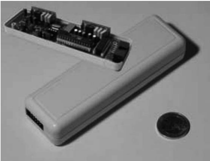
Figure 31.5 The new multisensor device consists of 2 two-axial accelerometers and a single-axial gyroscope. Assessed information (sampling frequency is 100 Hz) is processed by microcontroller that provides data to PC via RS232.
