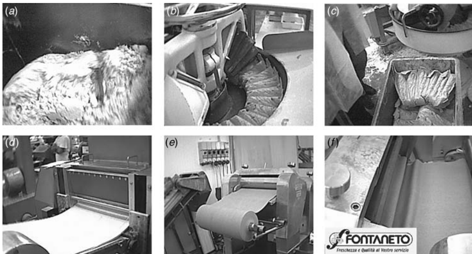
Figure 17.13 Artisanal fresh pasta-making process: mixing (a); dough kneading with gramola (b); dough cutting (c); intermediate dough sheeting (d); final sheeting (e); pasta after the first pasteurization (f). (Courtesy of Fontaneto, Italy).
