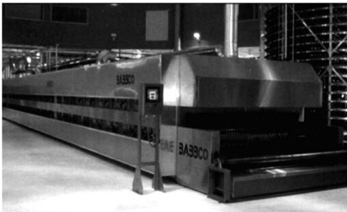
Figure 14.2 A direct heating oven. (Courtesy of C. H. Babb Co., Inc.)
