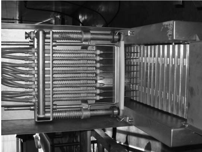
Figure 58.6 Picture of a typical brine injection machine with multineedle.
