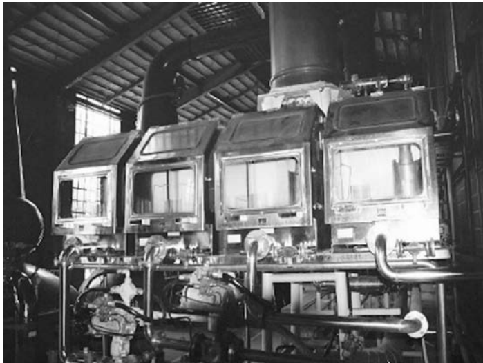
Figure 21.6 Monitoring of distillation as soon as vapors pass through the spirit safe.
