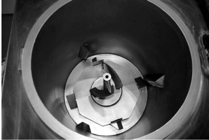
Figure 14.1 Interior of a Tweedy mixer (as typically used in the CBP). (Courtesy of APV Baker.)
