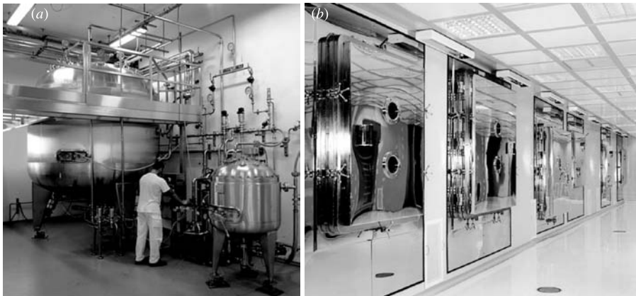
Figure 17.26 Production of starters: fermentation reactors (a), lyophilizers (b). (Courtesy of ANIDRAL, Italy).
