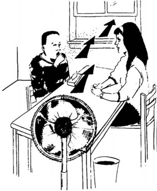
FIGURE 11.20 When two people sit across from one another, a fan can be positioned so that it blows air between the two people, directly toward an open window. If your fan oscillates back and forth, turn off that feature so that the fan always blows in the same direction. If you are buying a fan, make sure it can stay in the same position.
