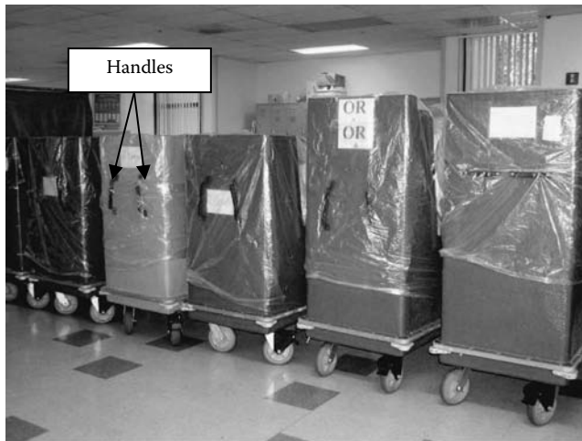
FIGURE 9.8 Comparison of the shorter and taller linen carts. Handles have been added for better grip.
