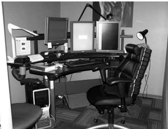
FIGURE 9.13 Radiology reading station with chair that adjusts for spine postures.
