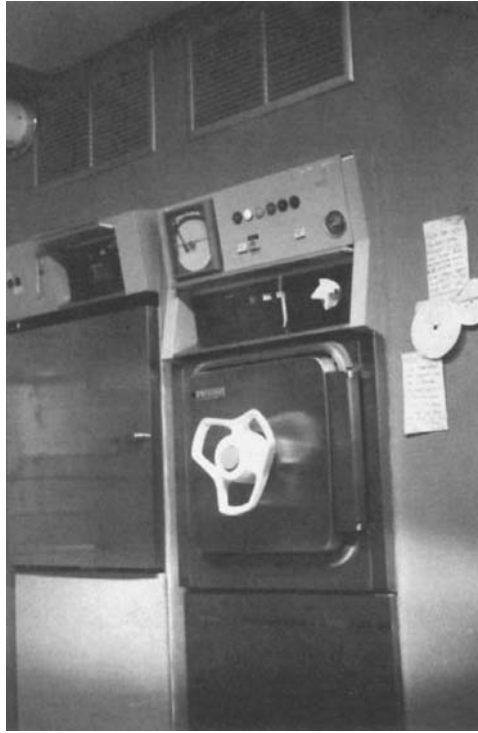
FIGURE 13.4 EtO sterilizer. Note the exhaust grill above sterilizer. This sterilizer also has a built-in Enviroguard system. (Photo by Frank Maniscalco.)
