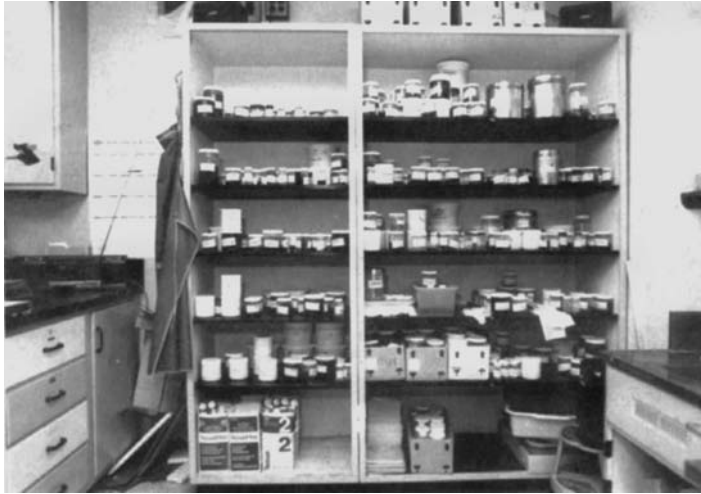
FIGURE 14.8 Specimen storage without enclosure or ventilation of formaldehyde. (Photo by Frank Maniscalco.)
