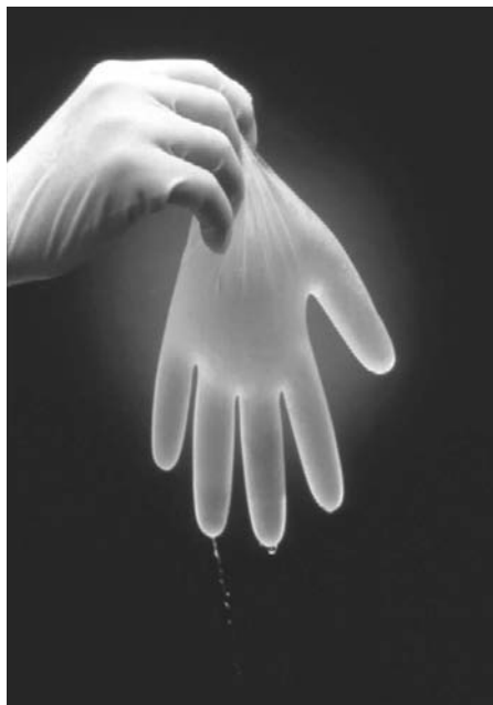
FIGURE 20.2 Following clinical- or simulated-use studies, fill the glove with water and observe for leaks.
