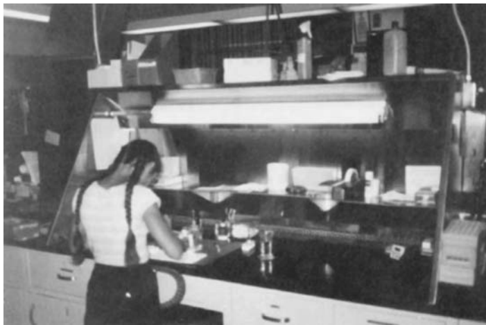
FIGURE 14.6 Slot-type hood for tissue mounting and specimen cutting. Notice the slot at the back of the hood. (Photo by Frank Maniscalco.)
