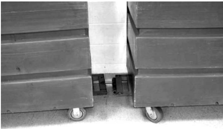
FIGURE 9.7 Hitch for joining linen carts.
