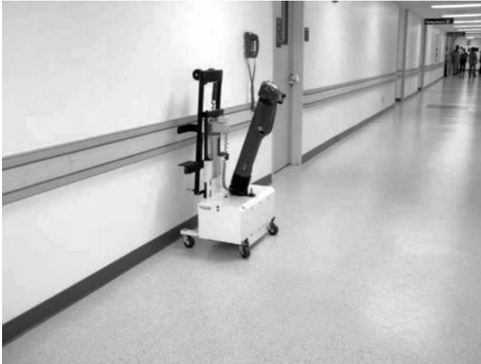
FIGURE 9.6 Motor for transporting carts.
