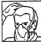
FIGURE 11.29 MOLDEX 2200 Fume, Dust Mist Respirator. Fitting instructions.
