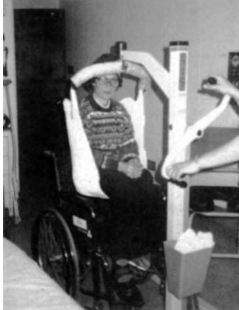
FIGURE 3.13 Ambulift C, has a semiadjustable base, a mechanical chain-winding mechanism for lifting/lowering with crank in vertical plane, and the sling attaches by loops and hooks.
