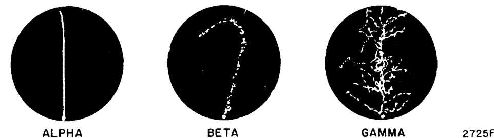
Figure 3-5. Cloud chamber photograph of alpha, beta, and gamma ray tracks. (J.B. Hoag: Electron and Nuclear Physics , courtesy D. Van Nostrand Co.) (H4)
