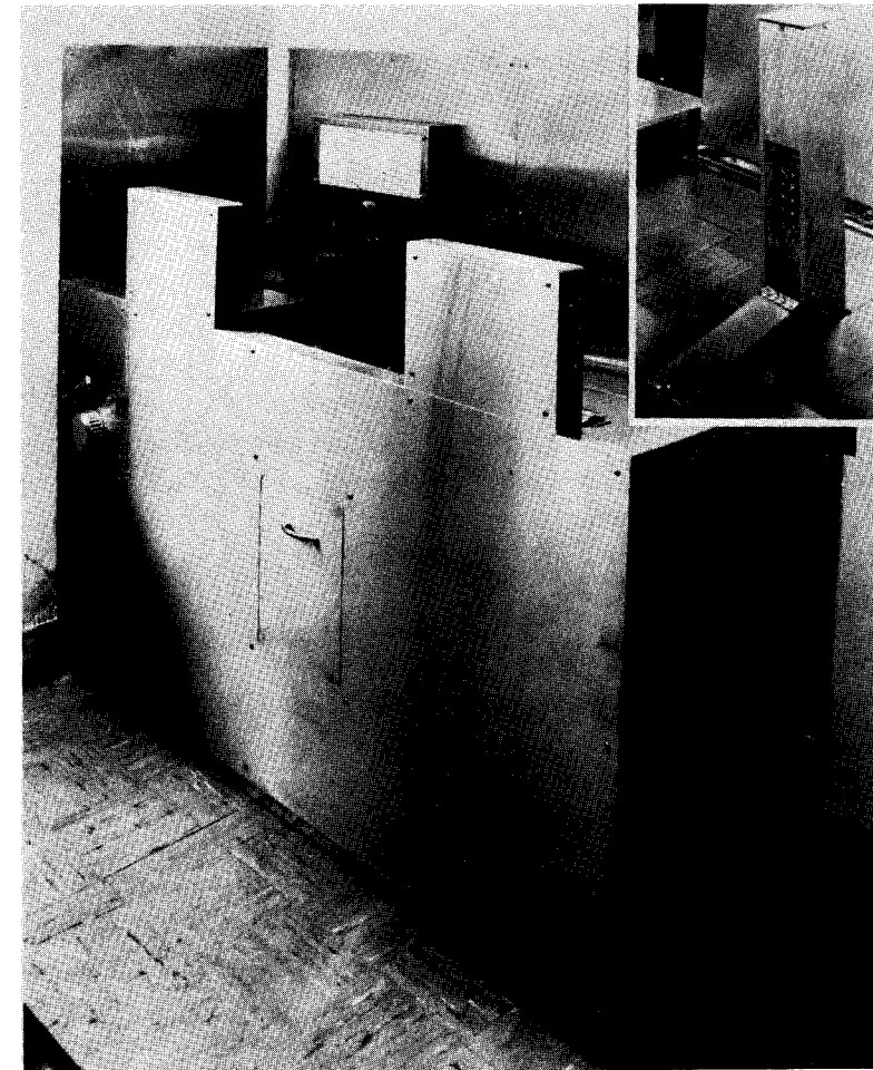
Figure 13-2. Photograph of radium safe and radium preparation surface in the Ontario Cancer Institute. Two barriers may be seen, behind which the technician may work. The insert shows the details of one of the drawers in its raised position. Lead glass eye shields may be added over each barrier if desired.
