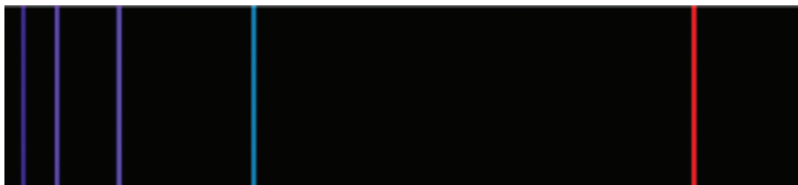
FIGURE 2.19 Emission spectrum of excited hydrogen. 18 The wavelengths of the colour lines are discussed in Chapter 13.
