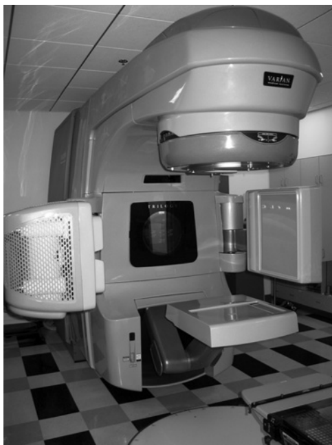
Figure 4-23 A modern dual-energy linear accelerator for radiation therapy.
