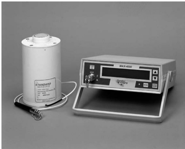
Figure 19-14 Well chamber and electrometer for measuring brachytherapy source strength. Source: Courtesy of Standard Imaging, Middleton Wisconsin.
