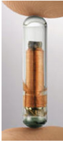
Figure 12-13 An electromagnetic transponder implanted in the region of a tumor to aid in localization.
