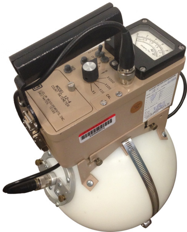
Figure 18-10 \text{BF}_3 proportional counter used for surveys of neutron levels.
