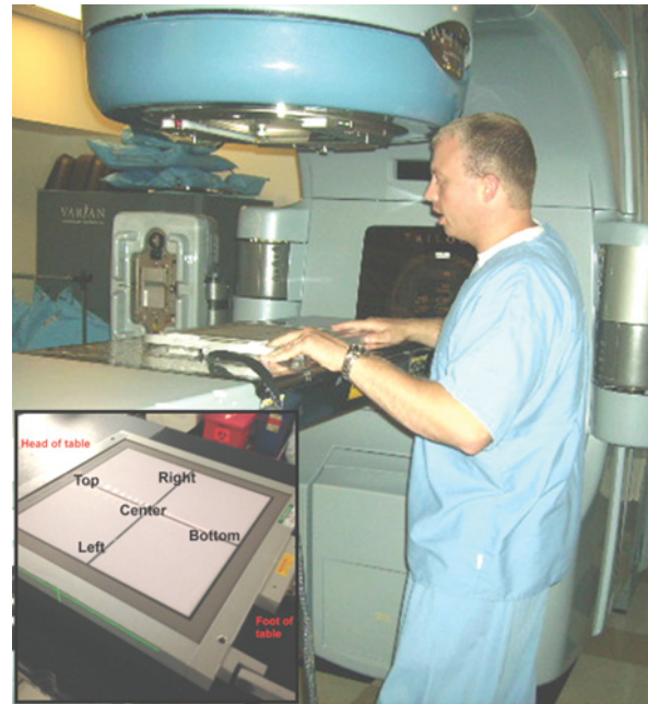
Figure 19-6 Daily beam measurements that readily measure beam output, flatness, and symmetry. The inset shows a beam's-eye-view and orientation of the device.
