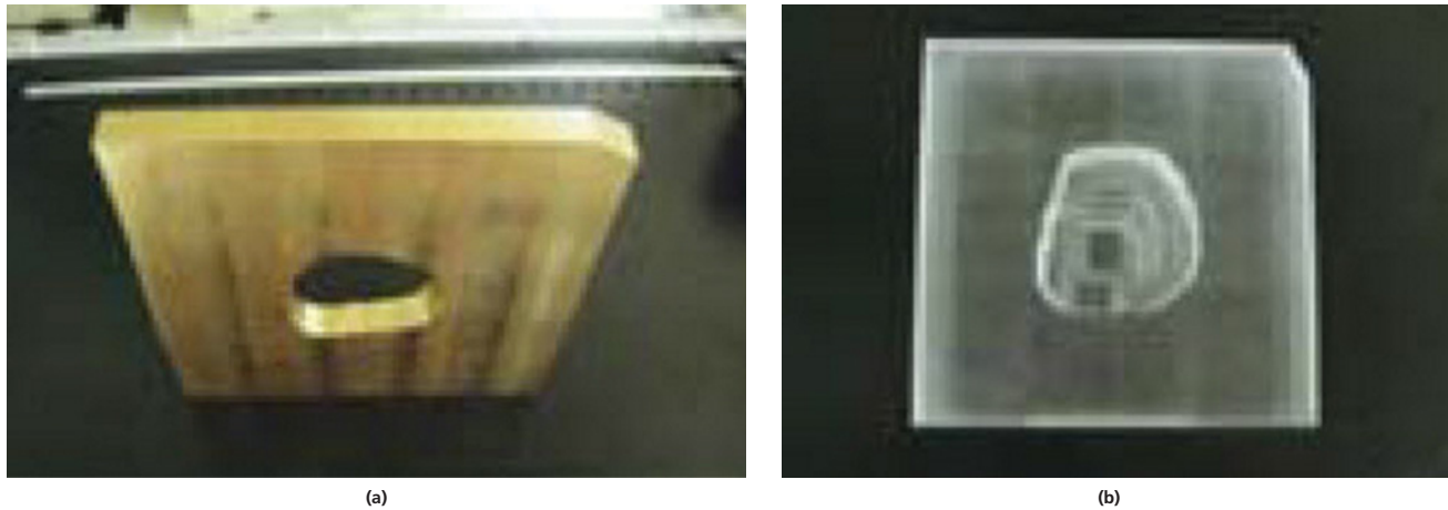
Figure 15-9 (a) Aperture and (b) compensator used for lateral and depth shaping of a proton beam.
