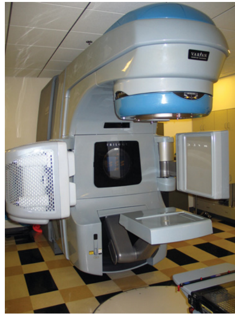
Figure 11-1 Gantry-mounted x-ray source (left in image) and image receptor (right in image) used in image-guided radiation therapy. The megavoltage image receptor is also shown in the bottom of the picture.
