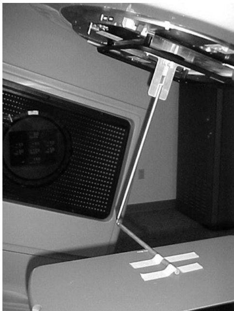
Figure 19-2 The use of mechanical pointers to measure the stability of rotation of the collimator, the gantry, and the patient treatment couch.
