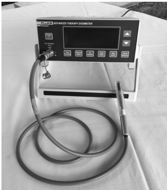
Figure 5-6 Integrated ionization chamber and electrometer used for radiation measurements irradiation therapy.
