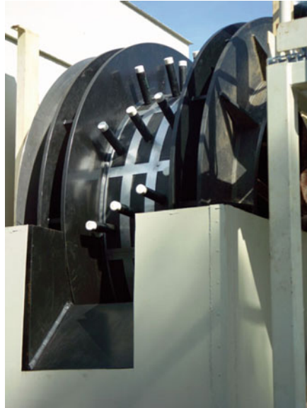
Fig. 6.17 Wheel equipped with rods for the transport of whole sugar beets
