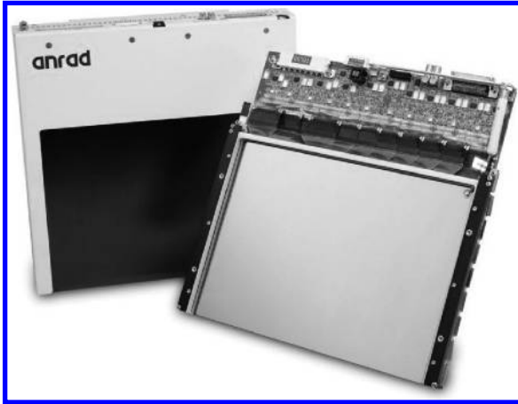
FIGURE 2.2 (See color insert.) Commercial a-Se semiconductor direct X-ray detector for full-field digital mammography. (From http://www.anrad.com/products-direct-x-ray-detectors.htm , Analogic, Direct Conversion X-ray Detectors, accessed August 12, 2013.)
