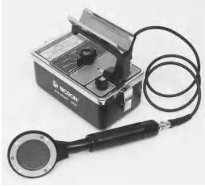
Fig. 12-10 Geiger counter with a thin "beta window."
