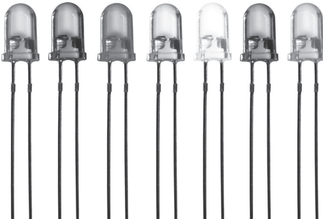
Figure 7.14 Light-emitting diodes. Different semiconductor properties produce different colors.
