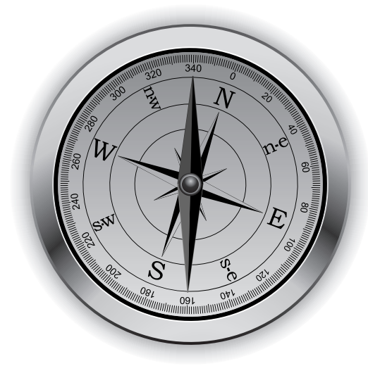
Figure 4.24 Compass north (magnetized needle) and true north (N) differ by about 20 degrees in Maine. The compass direction is closer to true north in most other parts of the United States.
