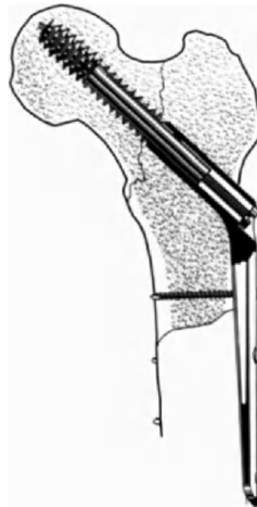
Figure 13-24. Illustration of hip nail on a fix fractured femoral head. Courtesy of DePuy, Division of Bio-Dynamics Inc., Warsaw, IN.
