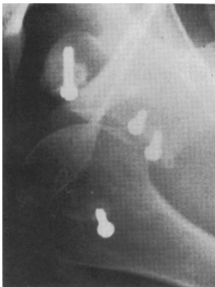
Figure 5-25. Mixed metals. Radiograph of a repaired shoulder. This patient experienced pain and disability. Examination of the screws following removal revealed one to be made of Co-Cr-Mo and the others of stainless steel. Reprinted with permission from Bechtol et al. (1959). Copyright © 1959, Balliere, Tindall, & Cox.
