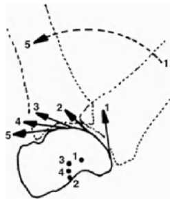
Figure 14-26. In this schematic view of the lateral ankle joint of a normal non-weight-bearing male, all of the instant centers are located within the talar body. Surface velocity shows the distraction at the beginning of motion with the subsequent sliding. Reprinted with permission from Sammarco et al. (1973). Copyright © 1973, W.B. Saunders.
