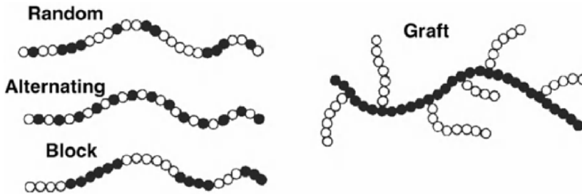
Figure 2-18. Possible arrangements of copolymers.
