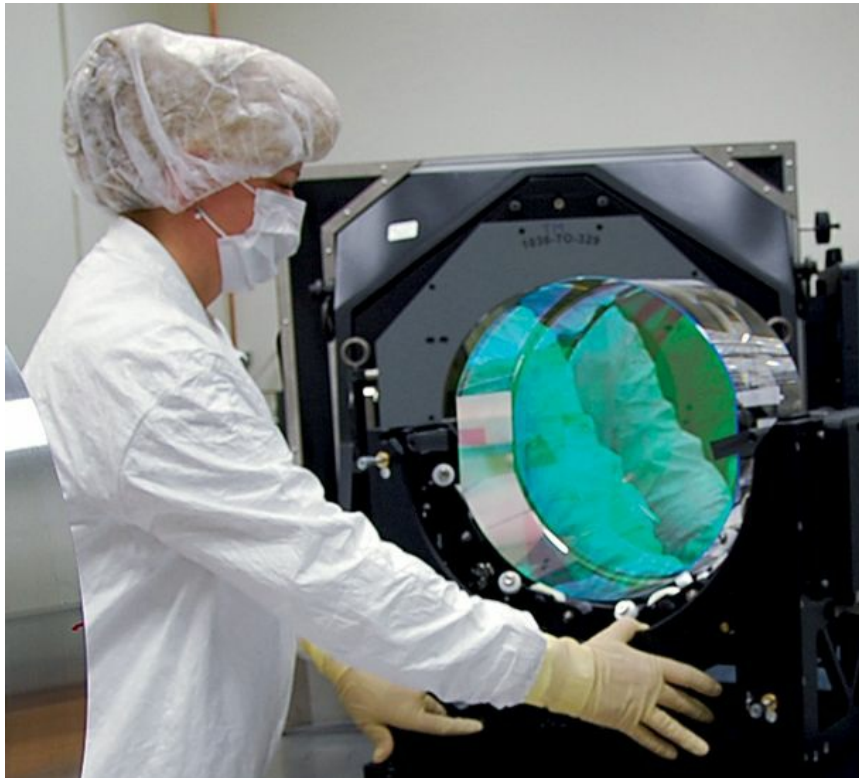
Fig. 26.2. A 40-kilogram mirror being prepared for installation in LIGO. Its location fluctuates, quantum mechanically, very, very slightly: one ten-billionth the diameter of an atom.
