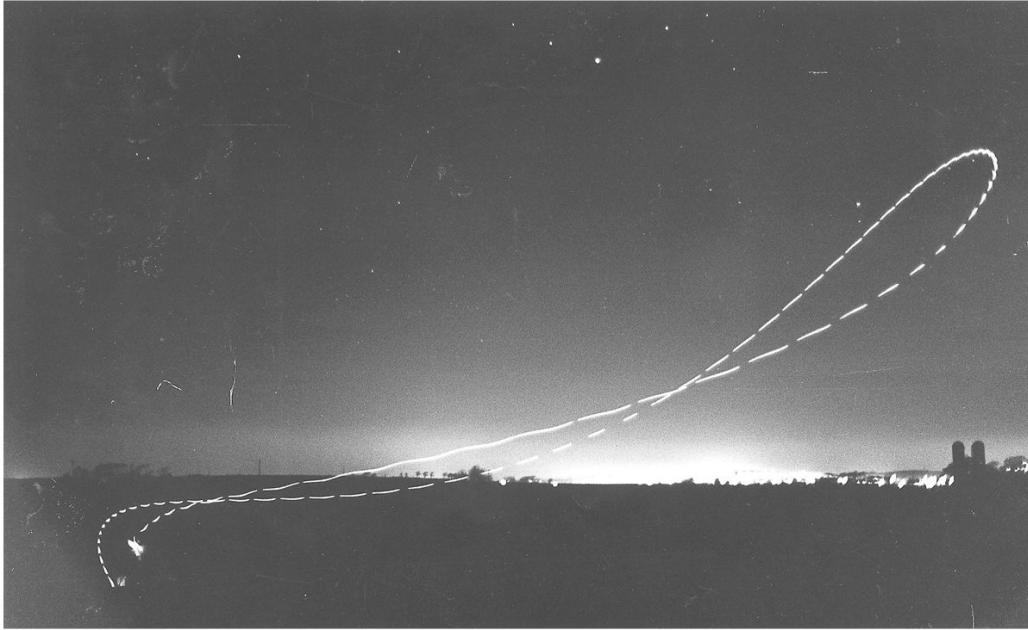
Figure 5.6: Time-Lapse Photograph of a Boomerang in Flight. The boomerang, thrown by Michael Hanson and photographed by Christian Taylor, was lit by a small battery-powered bulb at the tip.
