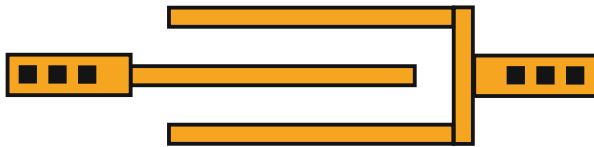
Fig. 5.7 Very small capacitors (<1 fF) are often realized inside one layer, this is a lay-out top view. For example, [82]
