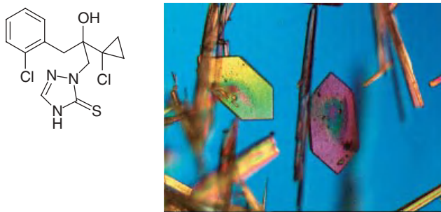
Figure 10.9 Concomitant polymorphs of prothioconazole (2004, Proline ® , Bayer CropScience) in plates and needle-like habit.
