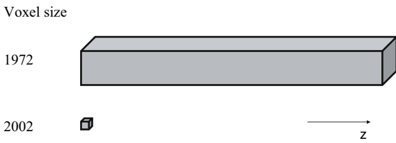
Fig. 2.2. Change in the size of a voxel element over the past 30 years
