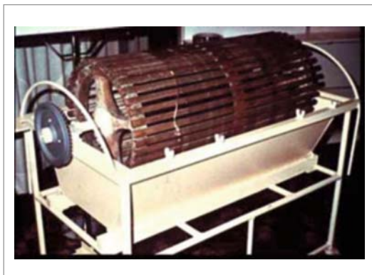
Figure 3-5. A picture of the rotating drum dialyzer invented by Kolff. (Cannot find copyright owner.)
