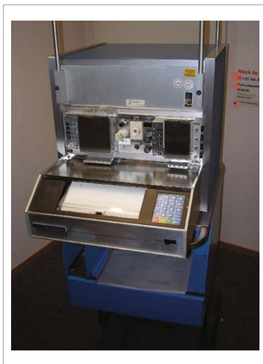
Figure 5-3. The Biostator dates from the mid-1970s and constituted one of the first attempts at a closed loop insulin pump. Glucose levels were measured on blood continuously withdrawn from an indwelling venous catheter. A computer with basic algorithms regulated the rate of delivery of insulin into a second catheter. Interestingly, it was the computer which was felt at the time to be the component which was unlikely ever to be miniaturized to the point at which a closed loop pump might become portable. (With kind permission of Prof Freckmann at the Institute of Diabetes Technology).
