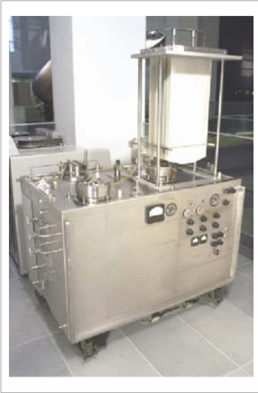
Figure 2-9. Screen oxygenator with 365 working parts.
