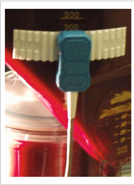
Figure 2-16. Level sensor that uses capacitance to detect level falling – will stop arterial pump.
