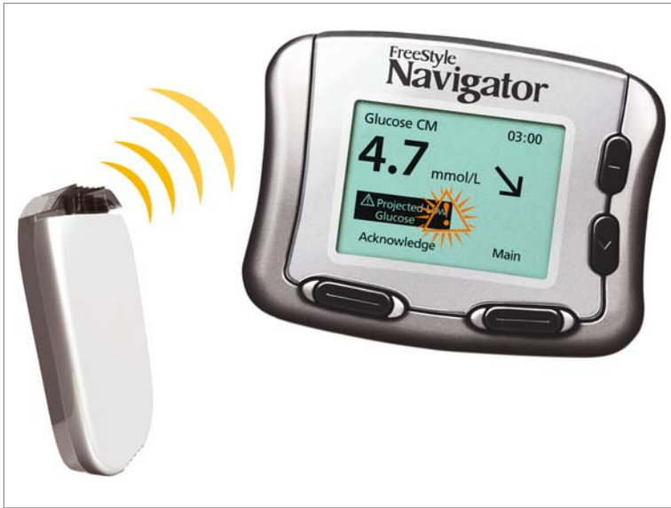
Figure 5-5. Abbott FreeStyle Navigator. The small unit on the left is attached to the skin and covers the electrode itself. The tissue glucose concentration is transmitted to a hand-held unit which displays not only the actual glucose level but also the fact that it is falling and displays an alarm for a risk of impending hypoglycemia. Reproduced by kind permission of Abbott Diabetes Care.
