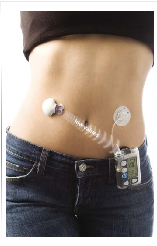
Figure 5-6. Medtronic MiniMed Paradigm Real-time monitor with MiniLink. The sensor has been inserted into the subcutaneous tissue in the right iliac fossa. This patient is also wearing a paradigm insulin pump infusing insulin continuously via the tubing and a cannula into the subcutaneous tissue of the left iliac fossa. Tissue glucose levels, transmitted from the sensor via the MiniLink, are collected in the pump which displays not only the actual tissue glucose levels but also the rate of change. At this stage, insulin delivery rates cannot be regulated by sensor glucose data. Reproduced by kind permission of Medtronic Ltd.
