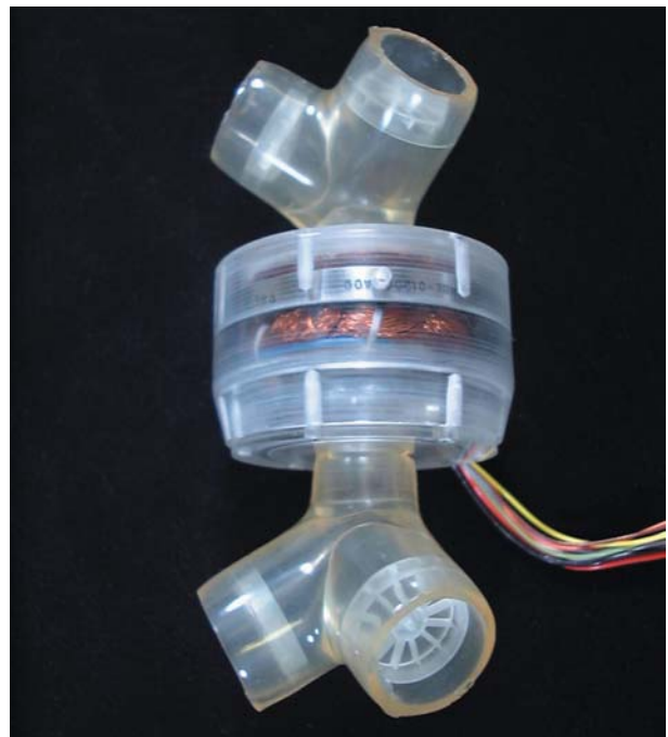
Figure 2. Actual model of the flow-transformed pulsatile total artificial heart.
