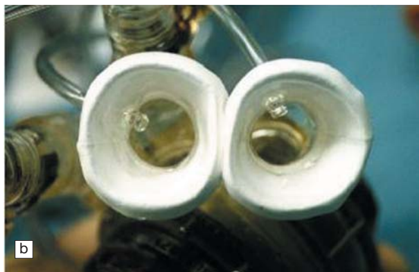
Figure 9. Atrial cuff model 9. L/R separate, D=38\text{mm} , h=18\text{ mm} , a=30^\circ (L), 40^\circ (R). (a) blood pump side view; (b) atrium side view.
