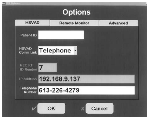
Figure 7. Clinical User Interface option to enable remote monitoring and control via telephone lines.
