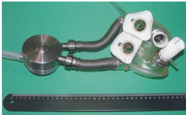
Figure 2. Intrathoracic pumping unit of the electrohydraulic total artificial heart system. The unit is composed of a blood pump subunit and an energy converter subunit consisting of a brush-less DC motor/regenerative pump assembly.
