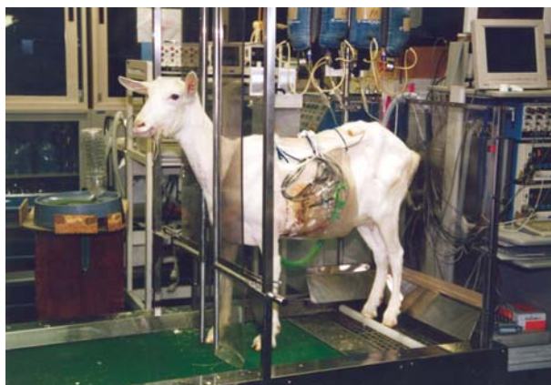
Figure 3. The goat that survived for 46 days with the UPTAH (at 31 days).
