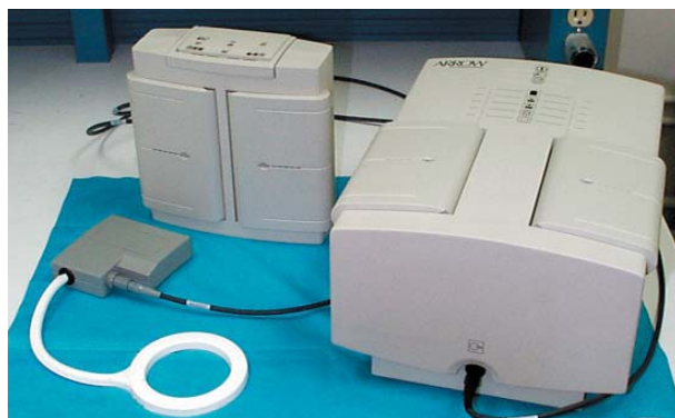
Figure 4. External electronics. Power Transmitter (lower left), Power Pack (upper left), and battery charger.
