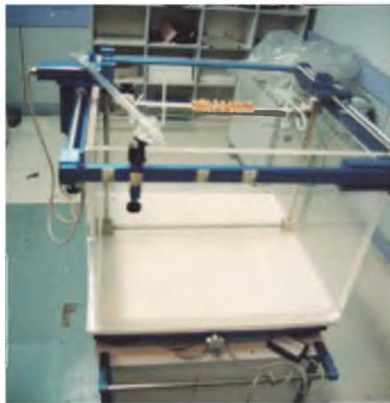
Figure 3.9 A needle cover tube (NCT) array mounted in an RFA guide rail for irradiation.
