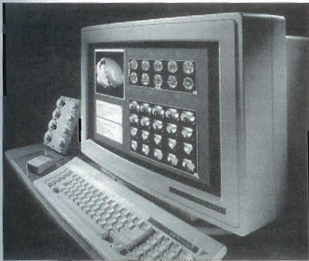
Figure 4-22 Workstation with windows environment provides the ability to perform several processes simultaneously. The mouse is used to move the cursor between windows for interaction with the different processes.
