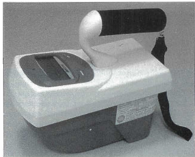
Figure 7-2 An ionization chamber is used to measure high exposure rates and is used for large sources of radioactivity and measures in mR/hr.
