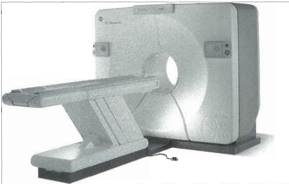
Figure 10-7 Dedicated bismuth germinate ring scanner containing 12,096 crystals that obtains 35 slices simultaneously.
