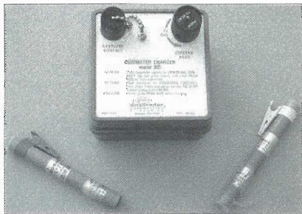
Figure 7-5 Pocket ionization chambers, seen as pencil-sized cylinders, are portable ion chambers. The pocket dosimeters are charged and reset to zero exposure setting while on the charger (seen in the center). Dosimeter may be read by looking through the lens in the end of the dosimeter to see the accumulated amount on the scale at any time.
