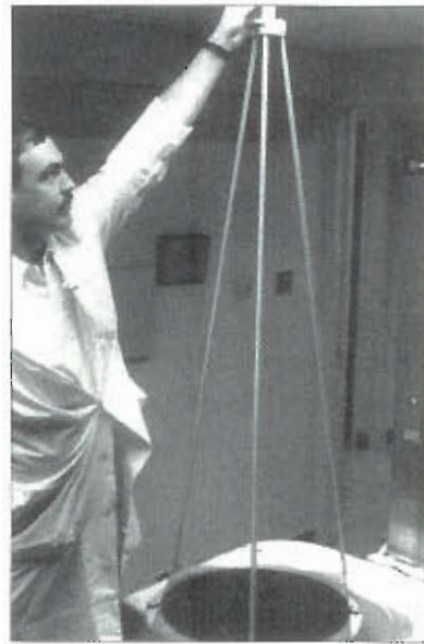
Figure 3-35 Tripod source receptacle used for intrinsic scintillation camera testing.
