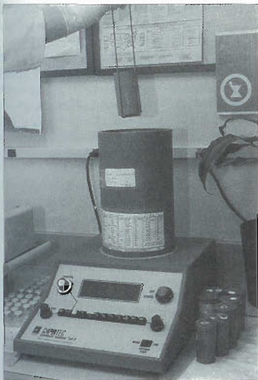
Figure 6-19 Molybdenum-99 assay chamber being placed in a dose calibrator.
