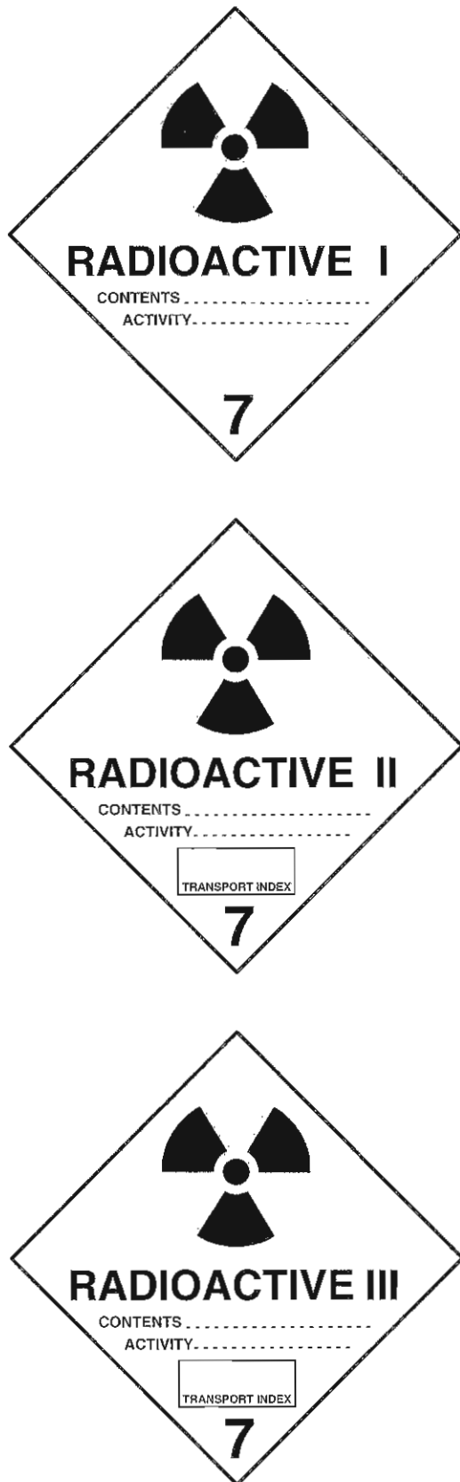
Figure 7-6 Transportation labels for radioactive materials: White I label, Yellow II label and Yellow III label. The number (I, II, or III) indicates the relative level of exposure from the radioactive package.
