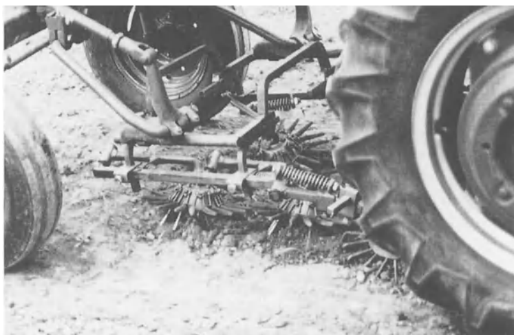
Fig. 9. Intra-row cultivator, Model C, made by Budding (United States).
