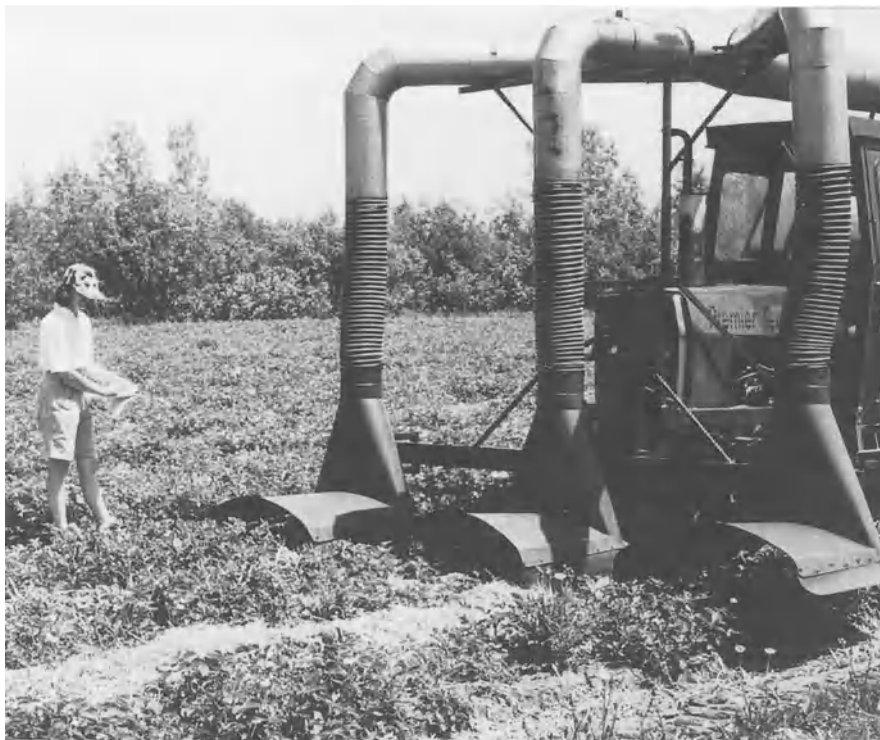
Fig. 1. Tractor-mounted Biovac in a strawberry field.
