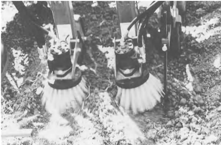
Fig. 2. Vertical-axis brush weeder manufactured by Svensk Ekologimaskin AB (Sweden).
