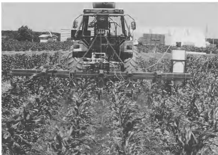
Fig. 1. Integrated mechanical and thermal weeding in row crops.
