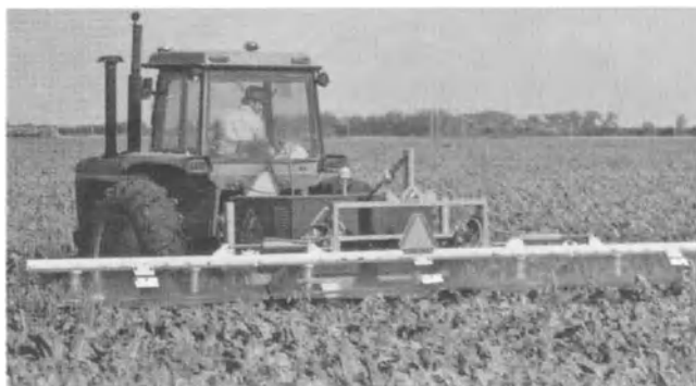
Fig. 1. Tractor-mounted electrical weed control machine, in operation.
