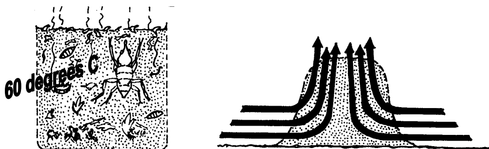
Fig. 9. Left: Temperatures of 60°C kill many soilborne disease organisms. Right: Steam rising during turning of a free-standing compost heap. Diagram©CSIRO (Handreck 1994).
