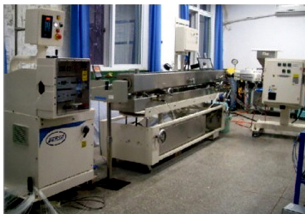
Figure 4 A typical catheter extrusion line. Courtesy: Elsevier Publications; G. Jin, M. Wang, D. Zhao, H. Tian, Y. Jin, Design and experiments of extrusion die for polypropylene five-lumen micro tube, J. Mater. Process. Technol 214 (1) (2014) pp. 50–59 [32].
