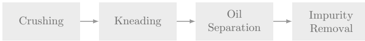
Fig. 1.4 Block diagram showing the main stages of the Virgin Olive Oil elaboration process
