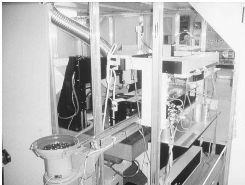
Figure 15 Photograph of a high-throughput protein excision and processing robot developed at the Centre for Proteome Research and Gene-Product Mapping in Australia and designed to automatically process two-dimensional gels or Western blots.
