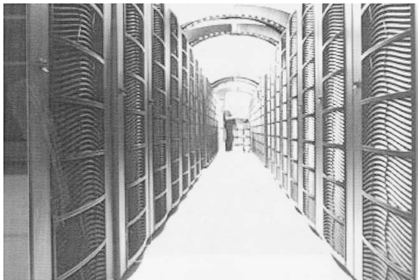
Figure 48 The other end of a cost-effective, high-performance computing infrastructure, namely a pre-existing infrastructure at national supercomputing facility, SARA, located in Amsterdam and connected to internal computing infrastructure (Fig. 47) by an experimental broad-band, optical-fiber link with a dedicated extension over 10 km. Pictured is the TERAS supercomputer consisting of two SGI Origin 3800 512 CPU systems with a maximum performance of 1Tflop per second. This is the latest upgrade among numerous other computing and storage solutions offered ( www.sara.nl ).
