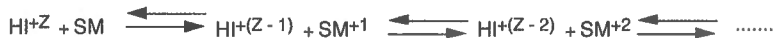
Fig. 14.26 Schematic diagram of charge exchange between a heavy ion and the stopping medium. The dots to the right of the figure are meant to indicate that the exchange reactions can proceed to lower ionic charges on the heavy ion.
