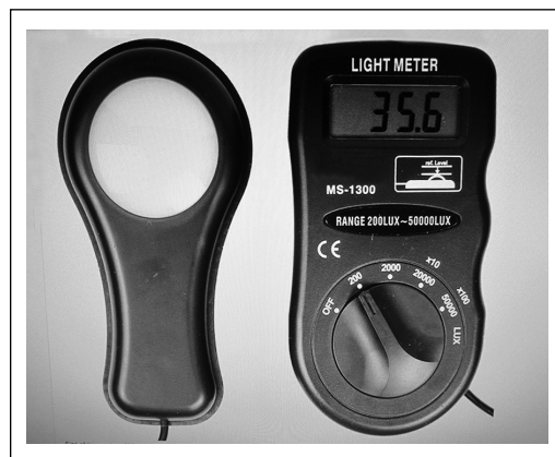
Figure 12-17. The photometer measures the brightness of light output from a display monitor. Readout units can be in lux , lumens or candela per square meter . (From Q. B. Carroll, Radiography in the Digital Age , 3rd ed. Springfield, IL: Charles C Thomas, Publisher, Ltd., 2018. Reprinted by permission.)
