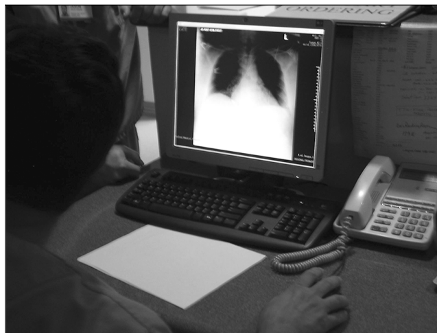
Figure 12-2. A typical display station consists of a low-resolution monitor with no capability for making permanent changes to images. (From Q. B. Carroll, Radiography in the Digital Age , 3rd ed. Springfield, IL: Charles C Thomas, Publisher, Ltd., 2018. Reprinted by permission.)
