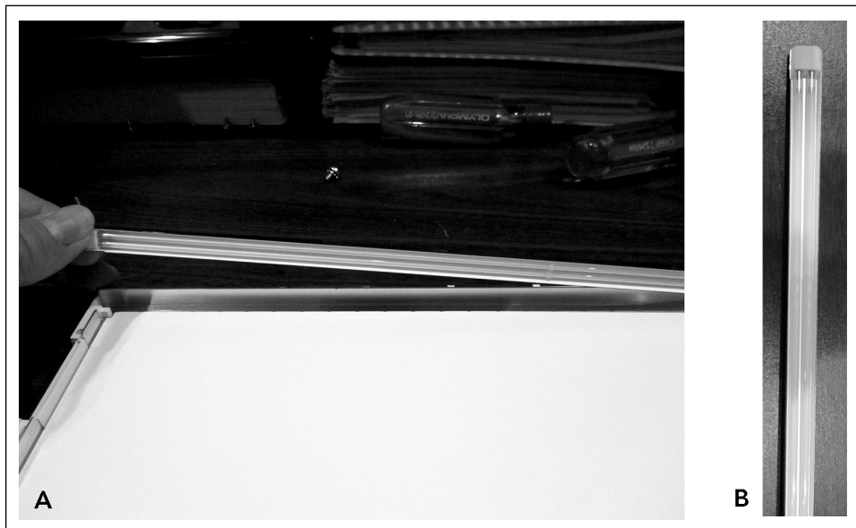
Figure 12-13. A pair of thin fluorescent light bulbs supply this LCD monitor with all the light it needs from a single side of the screen, A . Both bulbs can be better seen in a close-up photo, B . (From Q. B. Carroll, The Electronic Image: Display and Quality (video). Denton, TX: Digital Imaging Consultants, 2017. Reprinted by permission.)
