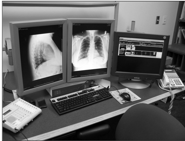
Figure 12-1. A radiologist's diagnostic workstation typically consists of two high-resolution (2000-pixel) monitors for image display, and an additional computer terminal with monitor for file management. (From Q. B. Carroll, Radiography in the Digital Age , 3rd ed. Springfield, IL: Charles C Thomas, Publisher, Ltd., 2018. Reprinted by permission.)
