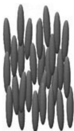
Figure 12-7. Nematic crystals are long, linear molecules that tend to align parallel to each other.
