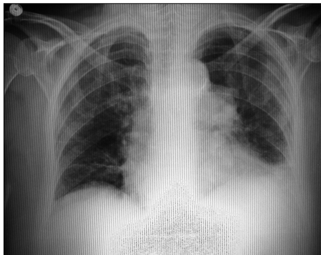
Figure 11-18. Aliasing (Moire artifact) caused by insufficient CR reader sampling of a high-frequency acquired image, resulting in false line patterns. (From Q. B. Carroll, Radiography in the Digital Age , 3rd ed. Springfield, IL: Charles C Thomas, Publisher, Ltd., 2018. Reprinted by permission.)
