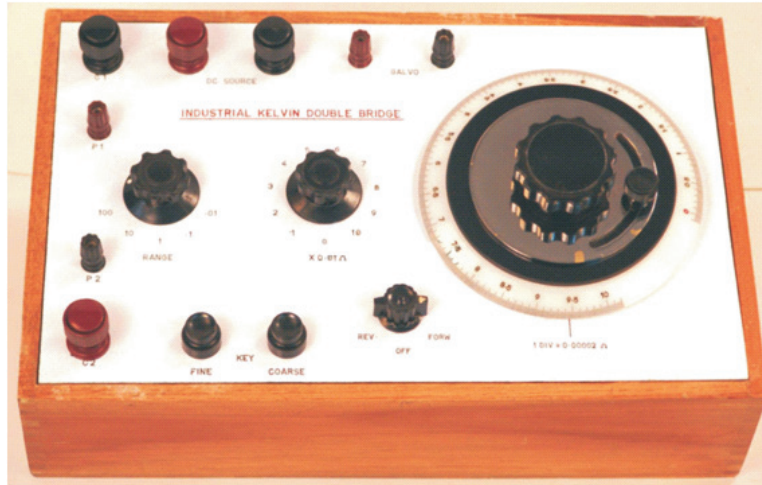
Fig. 4.8. Kelvin double bridge used in industry
