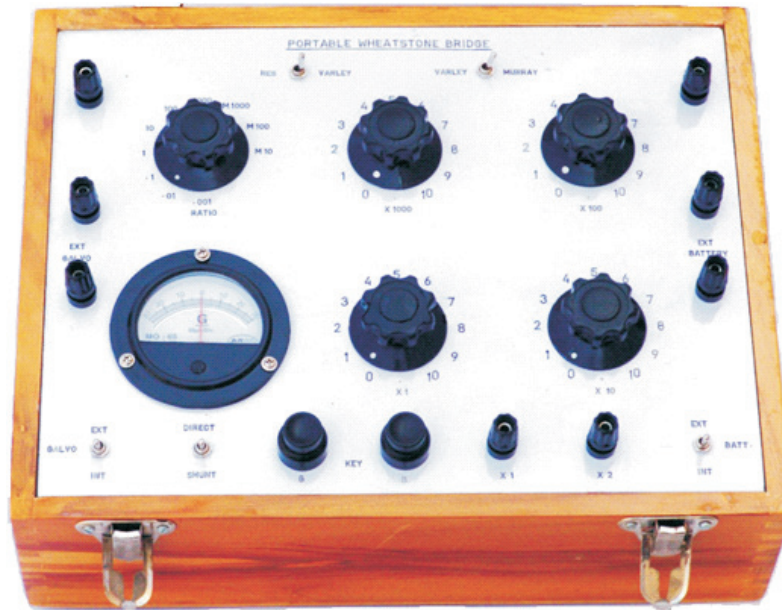
Fig. 4.15. Illustrating a portable Wheatstone bridge used in industry
