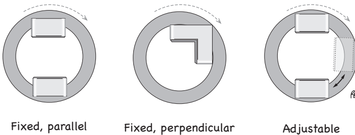
Figure 7.3 Configurations of two-headed SPECT camera.
