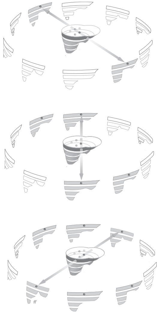
Figure 11.31 Nuclear medicine maximum intensity projection (MIP) image. The most intense feature (depicted by a dark gray sphere) along any ray is projected onto the MIP image.
