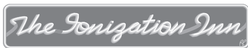
Figure 4.6 Continuous discharge. The voltage applied to a neon sign is high enough to generate spontaneous ionization that continues until the power is turned off.
