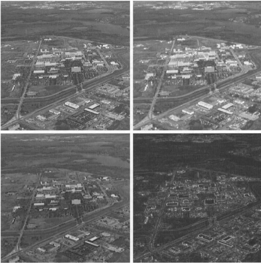
FIGURE 10.23 Dilation and erosion. (a) Original image. (b) Dilated image. (c) Eroded image. (d) Morphological gradient. (Original image courtesy of NASA.)
