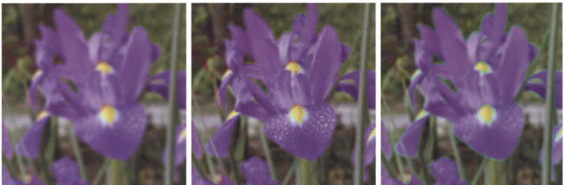
FIGURE 7.24 (a) Smoothed RGB image obtained by smoothing the R , G , and B image planes separately. (b) Result of smoothing only the intensity component of the HSI equivalent image. (c) Result of smoothing all three HSI components equally.
