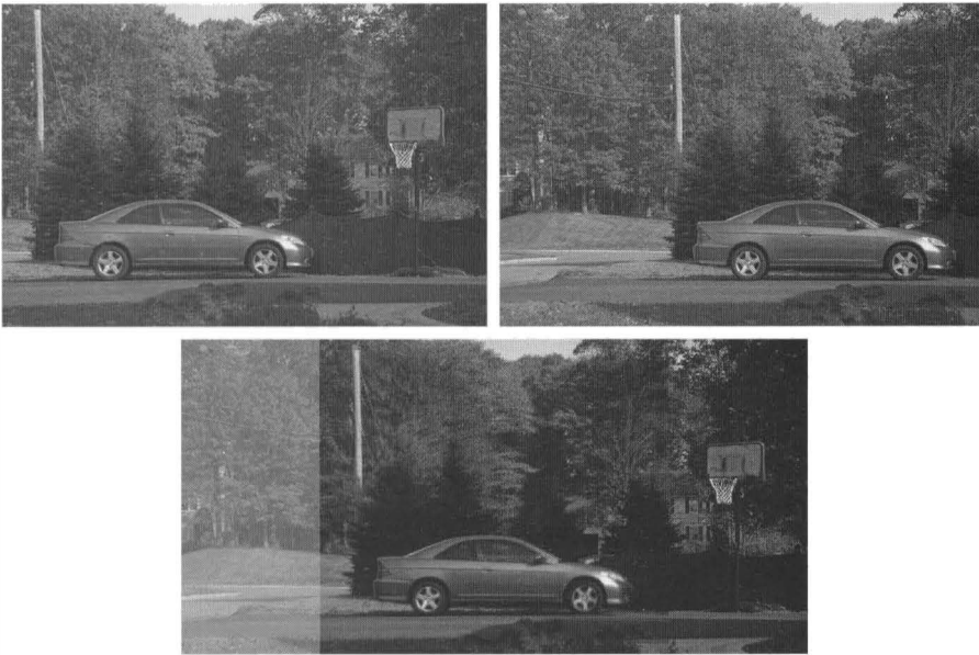
FIGURE 6.21 Using normalized cross-correlation to register overlapping images. (a) First image. (b) Second image. (c) Registered images as displayed using visreg .
