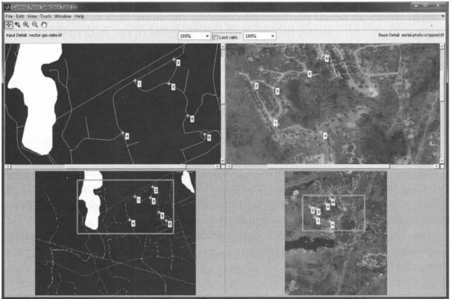
FIGURE 6.18 Selecting and matching features using the Control Point Selection Tool ( cpselect ). (a) Binary image showing road and other data. (Original image courtesy of Office of Geographic and Environmental Information (MassGIS), Commonwealth of Massachusetts Executive Office of Environmental Affairs.) (b) Aerial photograph of the same region. (Original image courtesy of the USGS National Aerial Photography Program.) (c) Screen shot of the Control Point Selection Tool.
