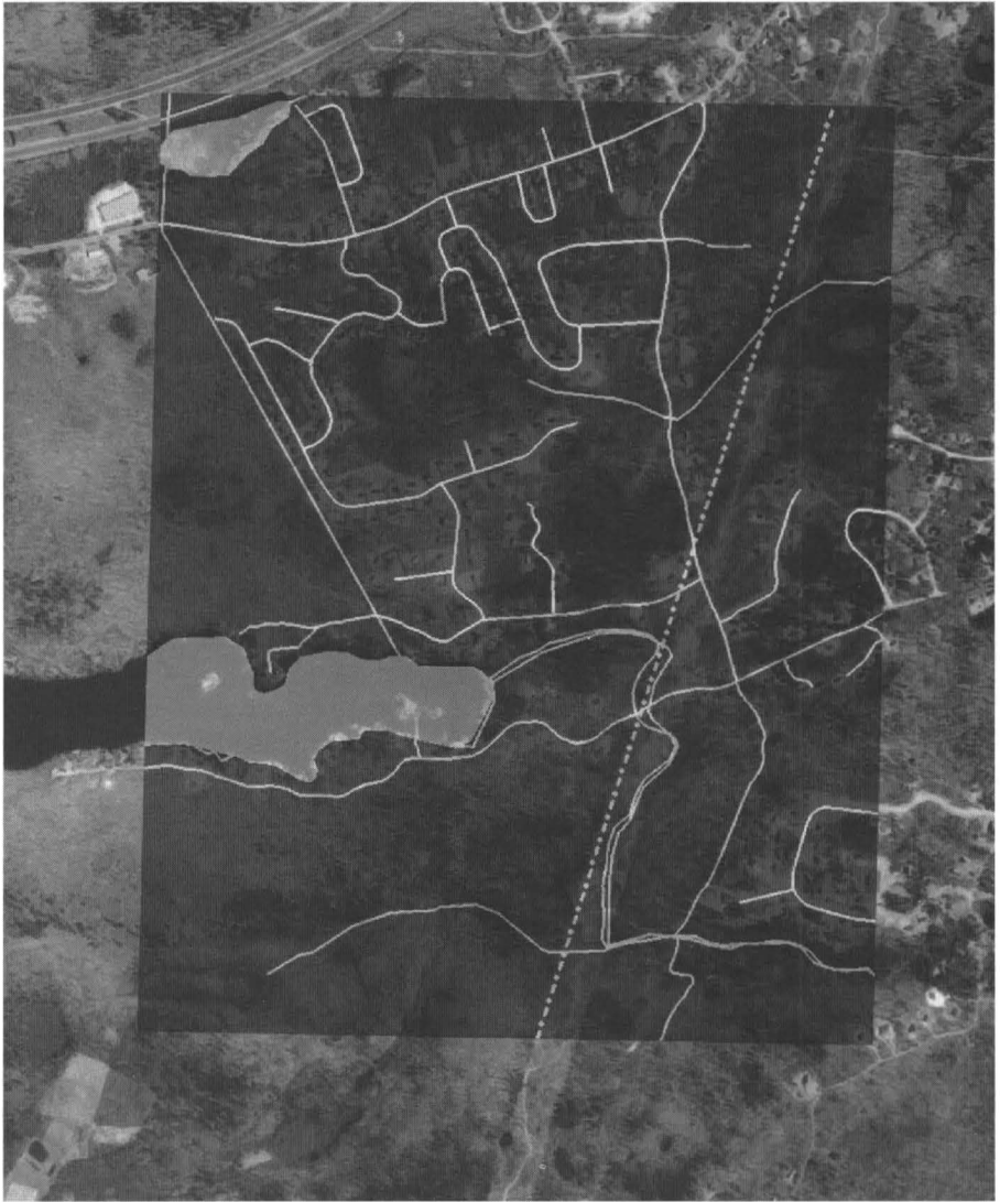
FIGURE 6.19 Transparent overlay of registered images using vis reg. (Note: the overlaid image was thickened using dilation to enhance its visibility. See Chapter 10 regarding dilation.)
