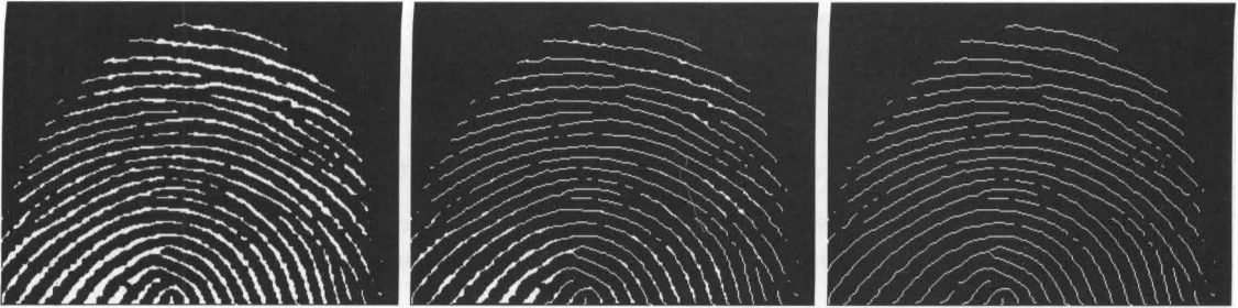
FIGURE 10.15 (a) Fingerprint image from Fig. 10.11(c) thinned once. (b) Image thinned twice. (c) Image thinned until stability.
