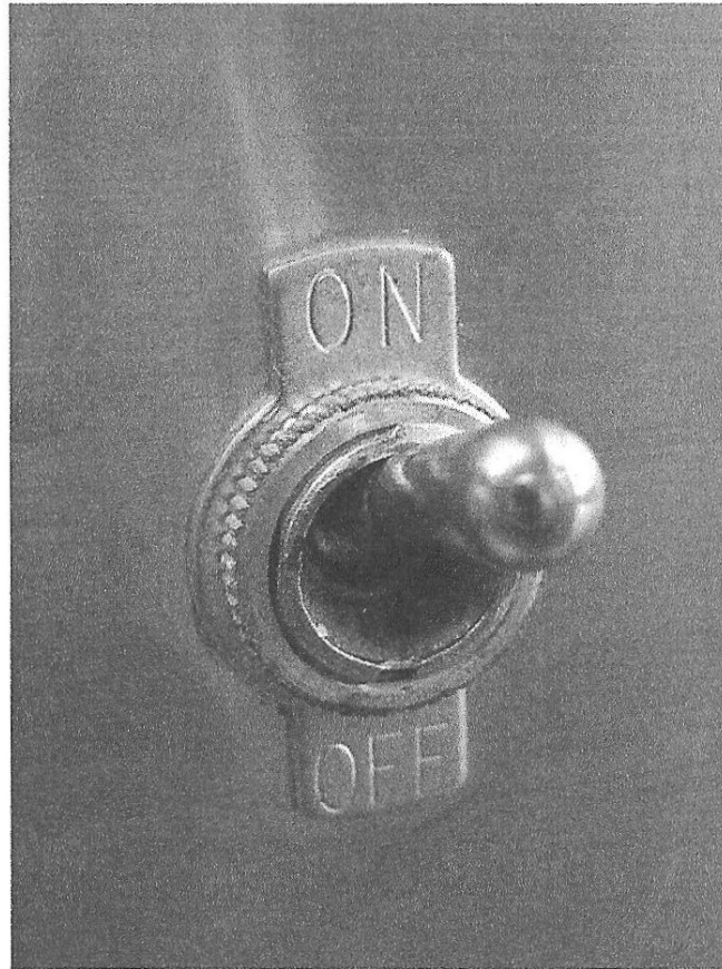
Figure 4.2 An electrical switch, a stand-in for two-valuedness: on/off \equiv 0/1. Jason Zack < http://en.wikipedia.org/wiki/File:On-Off_Switch.jpg >.
