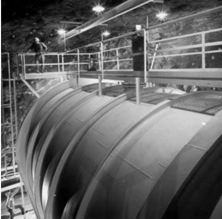
Figure 11.1 The Homestake Mine's chlorine detector, which Ray Davis Jr and colleagues operated for over three decades.
