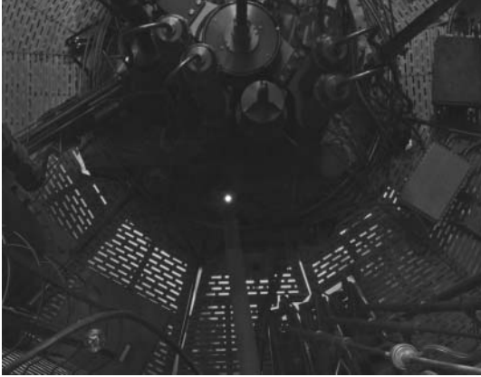
Figure 17.2 Top view of the central part of the high flux reactor of Institut Laue-Langevin seen through 7.5 m of light water. The heavy water tank in the middle is surrounded by a light water pool. The bottom of the latter is “illuminated” by Cherenkov light. The bright point below the center of the image is the V4 thimble tube, providing at its bottom a thermal neutron flux of 1.5 \times 10^{15} \text{ cm}^{-2} \text{ s}^{-1} . It can be manually loaded and unloaded with irradiation shuttles during reactor operation. (Photo U. Koster, ILL Grenoble).
