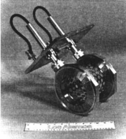
Figure 4.24 Capacitive pickup probes for time-of-flight measurement.
