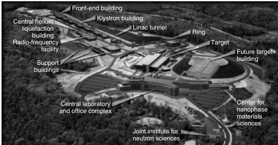
Figure 4.16 View of the ORNL SNS facility, indicating how the LINAC injects into the storage ring, from which the beam is extracted to the target.
