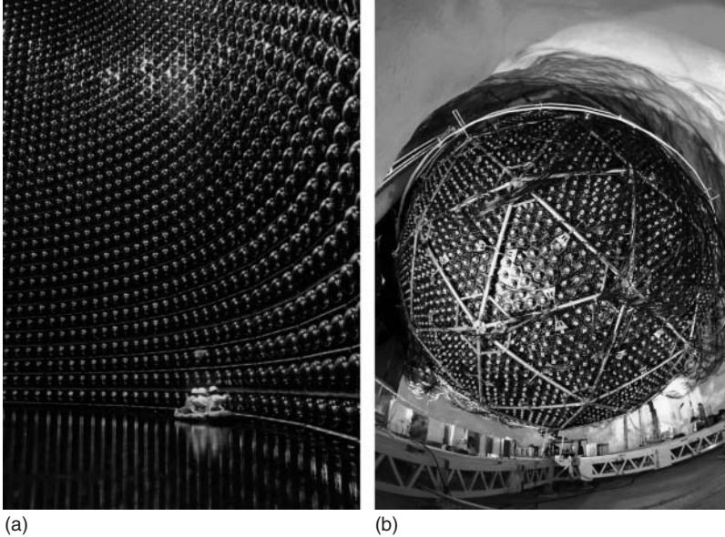
Figure 11.3 (a) The Super-Kamiokande detector during filling, with scientists cleaning photomultiplier tube (PMT) surfaces as the water rises. (b) Fish-eye photo of the SNO detector and cavity, showing the PMTs and support structure before cavity and detector filling.
