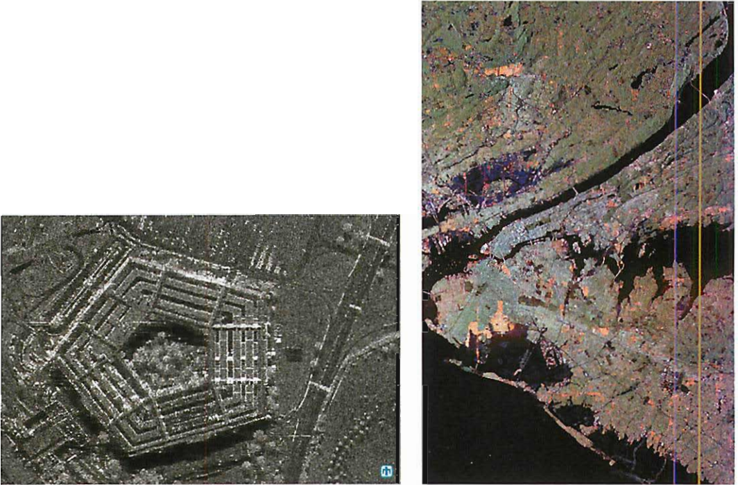
Figure 9.10 Radar images. These were taken using synthetic aperture radar (SAR). The image on the left is the Pentagon building in Washington, DC, and the image on the right is New York City.
