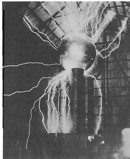
Figure 6.1 Large Van de Graaff generator at MIT. (Photo courtesy of U.S. Department of Energy.)
