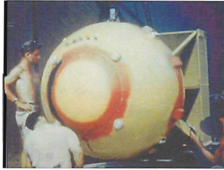
Figure 5.11 The plutonium implosion bomb that the United States dropped on Nagasaki. From the shape, you might guess that it contained a sphere of explosives. (Photo courtesy of U.S. Department of Energy.)
