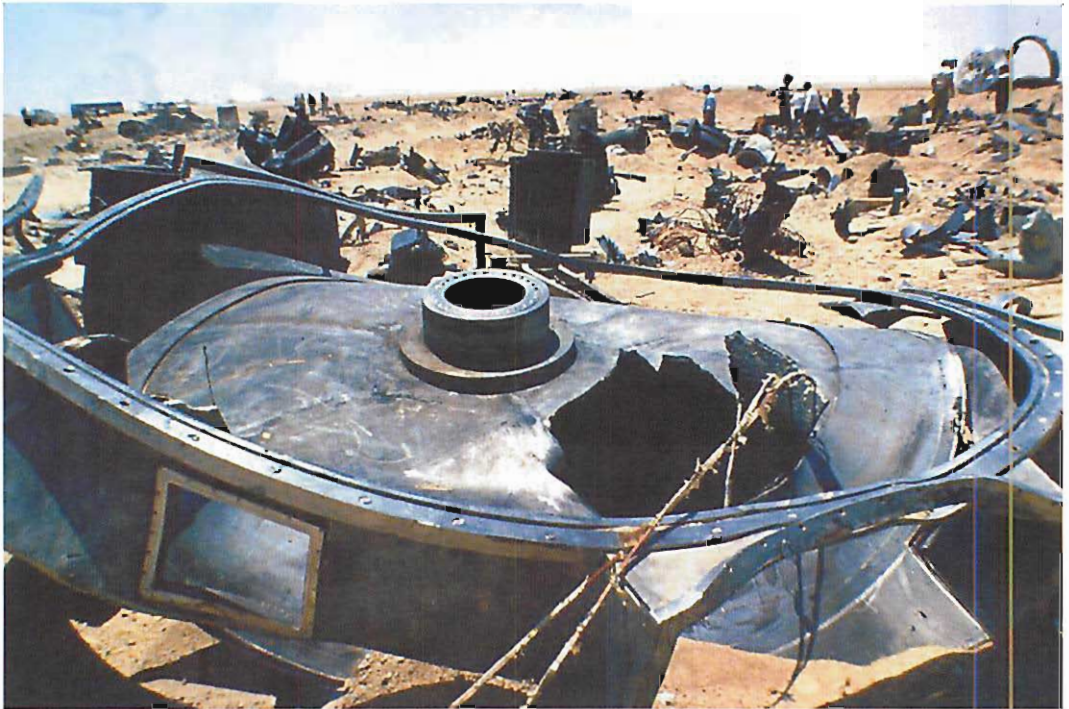
Figure 5.6 Iraqi Calutron. This field shows the pieces left after the International Atomic Energy Agency destroyed Saddam's Calutron. This Calutron had enriched uranium to 35% U-235; that was not yet enough to use for a bomb, but only a few more steps would have brought the enrichment to 90%. (Photo courtesy of U.S. Department of Energy.)
