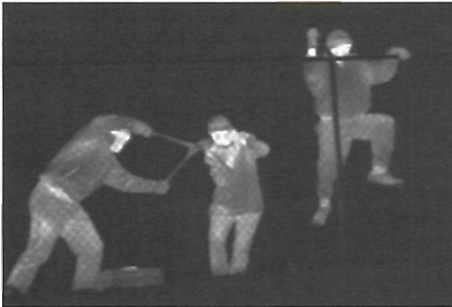
Figure 9.1 Infrared image of two people cutting a fence and one person climbing over. Notice that the warm parts of the image (face and hands) are brighter than the cooler clothing. (Copyright Indigio Systems, used with permission.)
