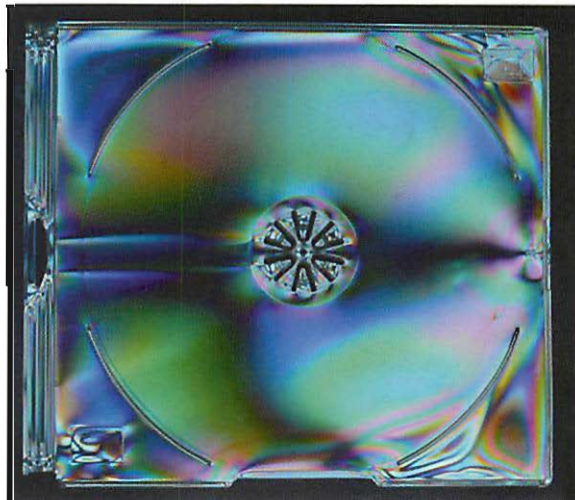
Figure 8.26 Plastic CD case, seen between two polarizers. Different colors show different amounts of stress left in the plastic when it was manufactured; black regions have little or no stress. You can see this in real life by crossing two pairs of polarizing sunglasses until no light gets through the combination (as in figure 8.25) and then putting a piece of stressed plastic between.
