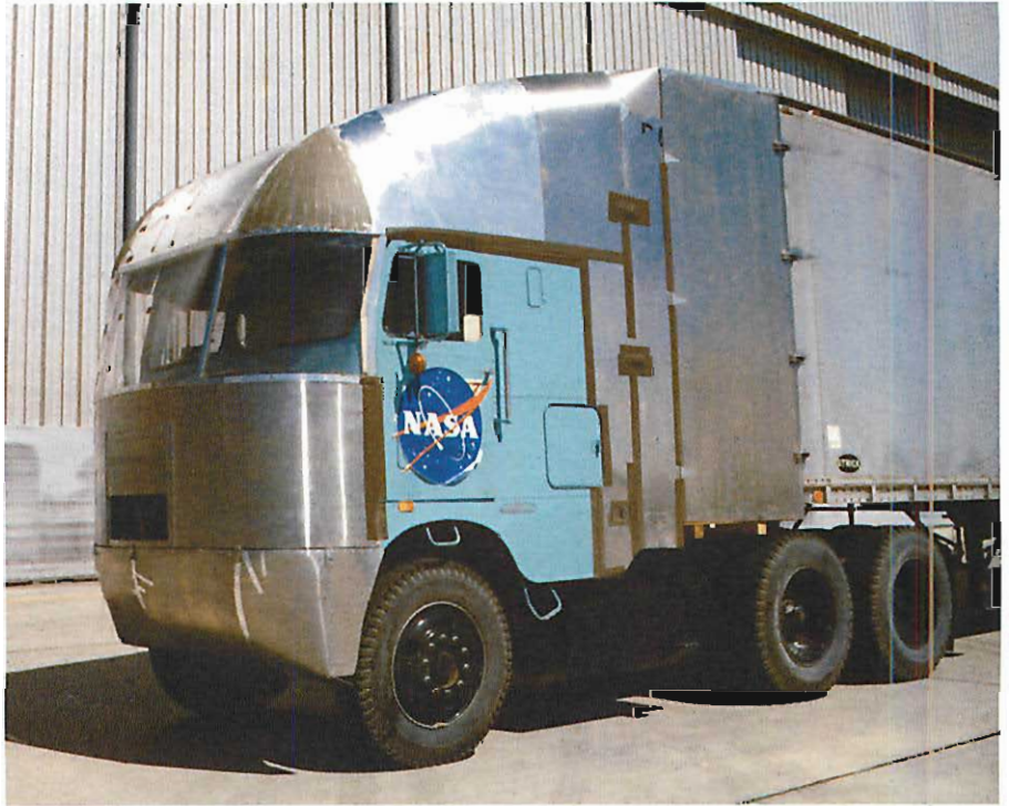
Figure 3.2 Truck with cab fairing to reduce air resistance. (Photo courtesy of NASA.)
