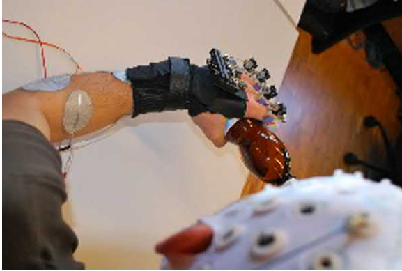
FIGURE 57.2 Example of a BMI for the restoration of grasping. The BMI is combined with functional electrical stimulation that activates the subject's peripheral nerves under the electrodes and contracts the corresponding muscles for hand closing and opening. This operation is further facilitated by the use of a light passive hand orthosis that synchronizes finger movements so as to generate natural grasping patterns. BMI, Brain-machine interface.
