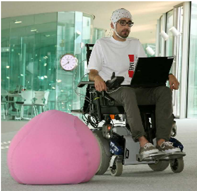
FIGURE 57.3 Brain-controlled wheelchair. Users can drive it reliably and safely over long periods of time thanks to the incorporation of shared control (or context awareness) techniques. This wheelchair illustrates the future of intelligent neuroprostheses that, as our spinal cord and musculoskeletal system, works in tandem with motor commands decoded from the user's brain cortex. This relieves users from the need to deliver continuously all the necessary low-level control parameters and, so, reduces their cognitive workload.
