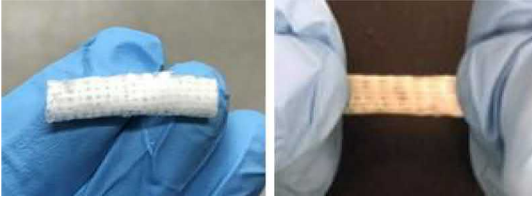
FIGURE 54.10 3D printed cylindrical tough mesh coated with hydrogel. 3D, Three-dimensional.
