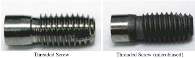
Fig. 5.13 Two threaded screws, one untreated and another treated with microblast, are shown
