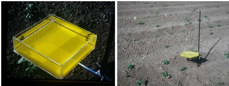
FIGURE 2.4 Yellow water pan trap used to trap aphids. Close up of trap (left) and deployed in the field (right).
