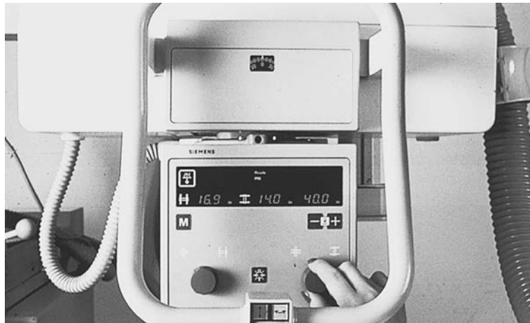
FIGURE 7-10 The x-ray field measurement guide on the front of a collimator.
