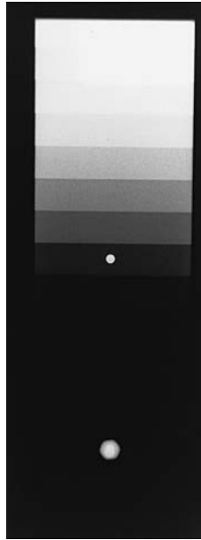
FIGURE 5-7 Radiograph of a penetrometer showing step-wedge densities.
