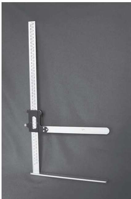
FIGURE 8-7 A caliper is used to measure part thickness.
