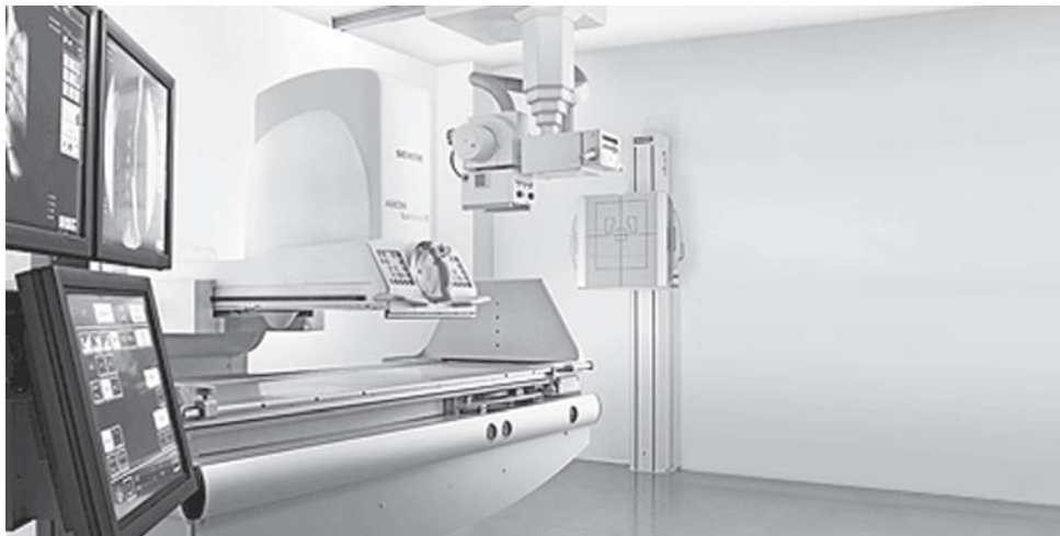
FIGURE 10-2 A typical radiographic and image-intensified fluoroscopic unit.
