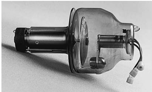
FIGURE 2-6 A glass envelope x-ray tube as it appears before installation in a tube housing.
