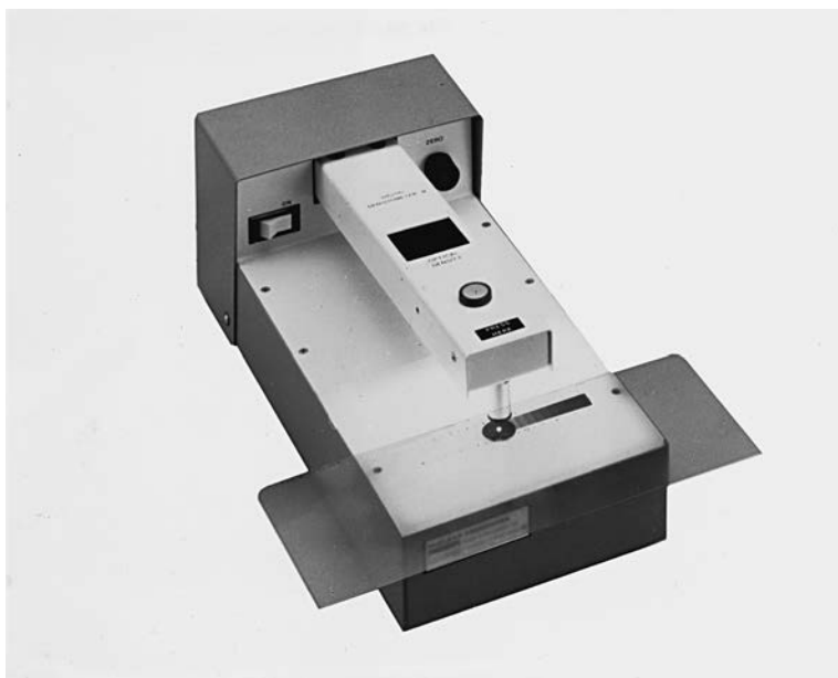
FIGURE 5-9 A densitometer is used to measure optical densities.
