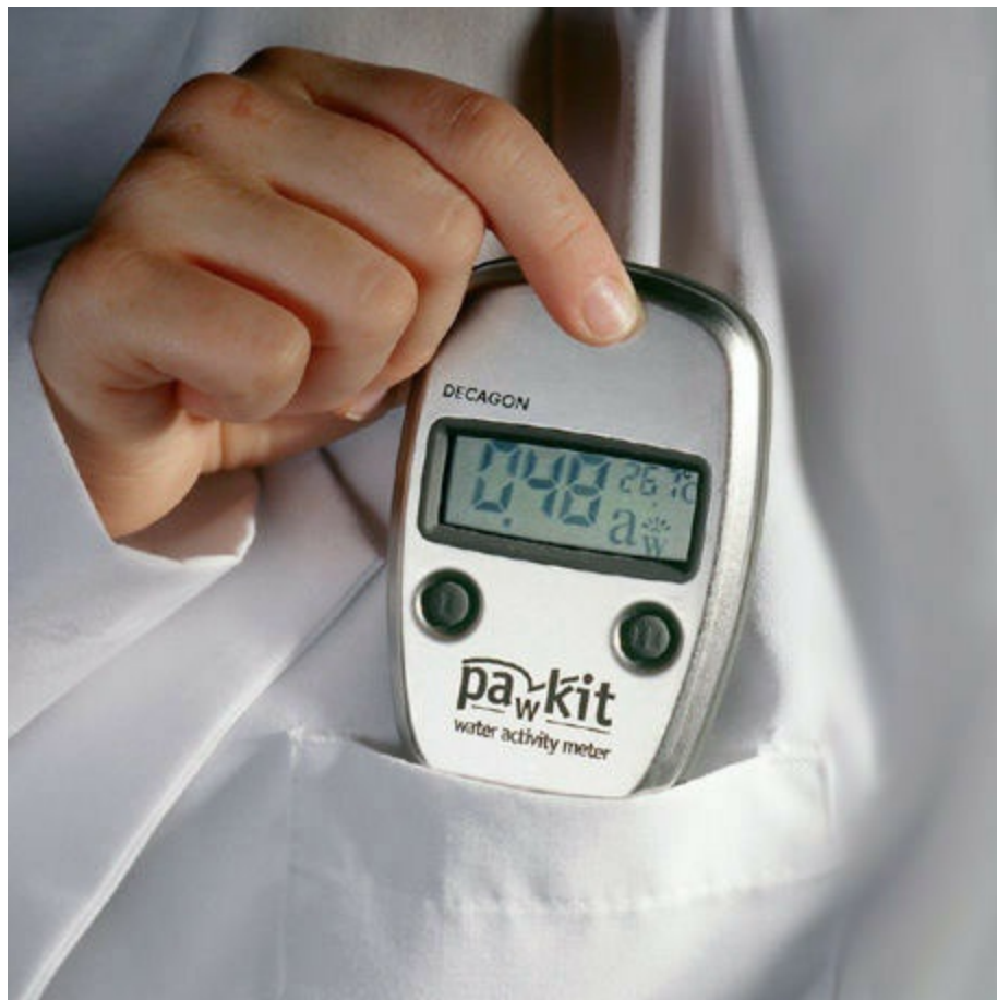
Photo 1.5 Originally designed for government inspectors, the 4-inch Pawkit is a reliable water activity instrument for use on-the-go. A push of a button brings an accurate reading within five minutes.
