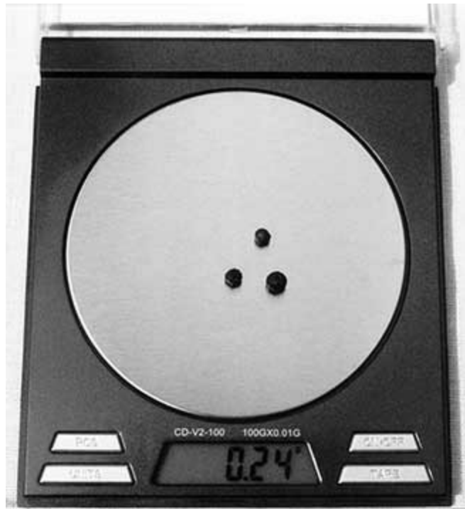
Photo 12.3 AWS Compact Digital Scale v2.0 by American Weigh Systems . Capacity: 100 g Accuracy: 0.01 g (0.001 oz)
