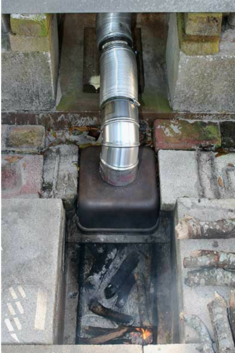
Photo 7.4 Burning whole logs of wood is a comfortable way of generating cold smoke when smoking continues for a long time.
