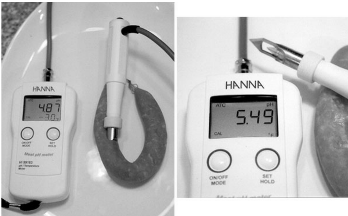
Photo 1.1 and Photo 1.2 HI 99163 Portable Meat pH Meter. Photo and information courtesy Hanna Instruments http://www.hannainst.com
