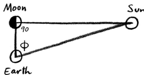
The right-angle triangle made by the Earth, moon, and sun when the moon is half full
