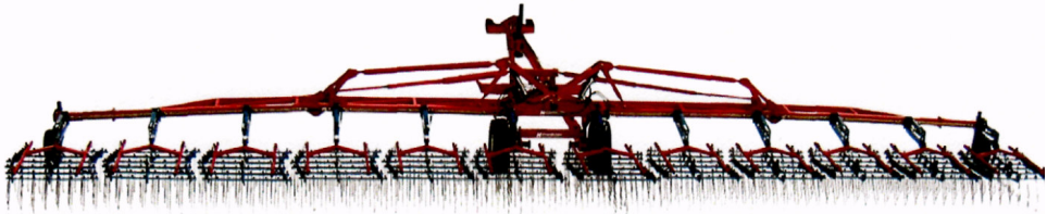
Figure 28. Ecological harrow: a means for post-sowing crop harrowing [32].
