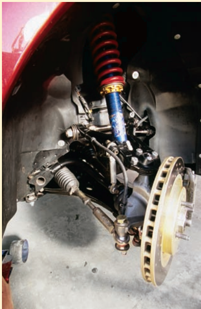
■ FIGURE 9.32 Typical automotive suspension system. © Transtock Inc./Alamy.
