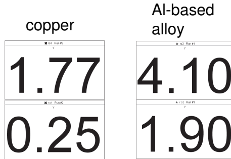
Fig. 12. Resistivity (in 10^{-8} \Omega \cdot \text{m} ) of copper and Al-based alloy at room (top) and liquid nitrogen (bottom) temperatures displayed by Digits .
