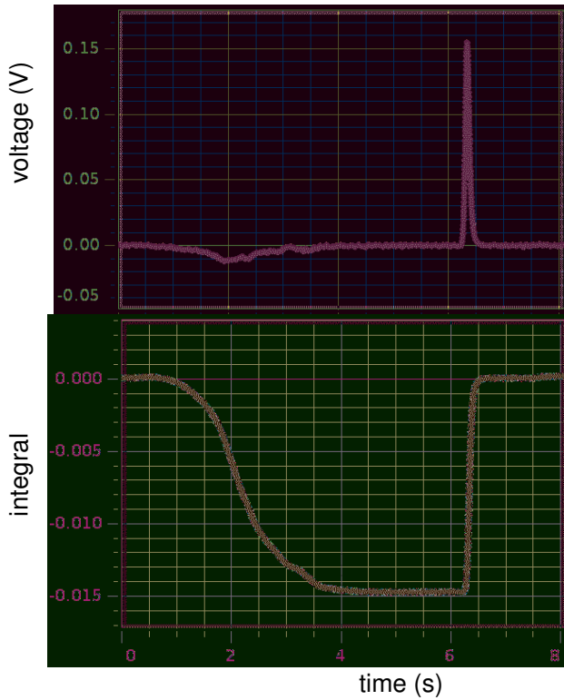
Fig. 2. Measurement data: voltage induced in the coil and the integral of the induced voltage.
