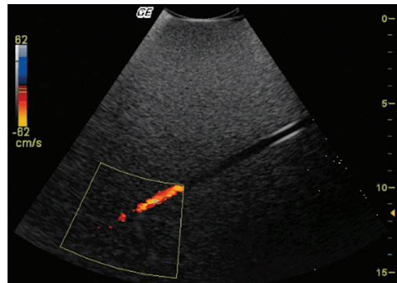
Fig. 11.16 Penetration depth measurement. The depth is measured at which the colour flow can no longer be distinguished.
