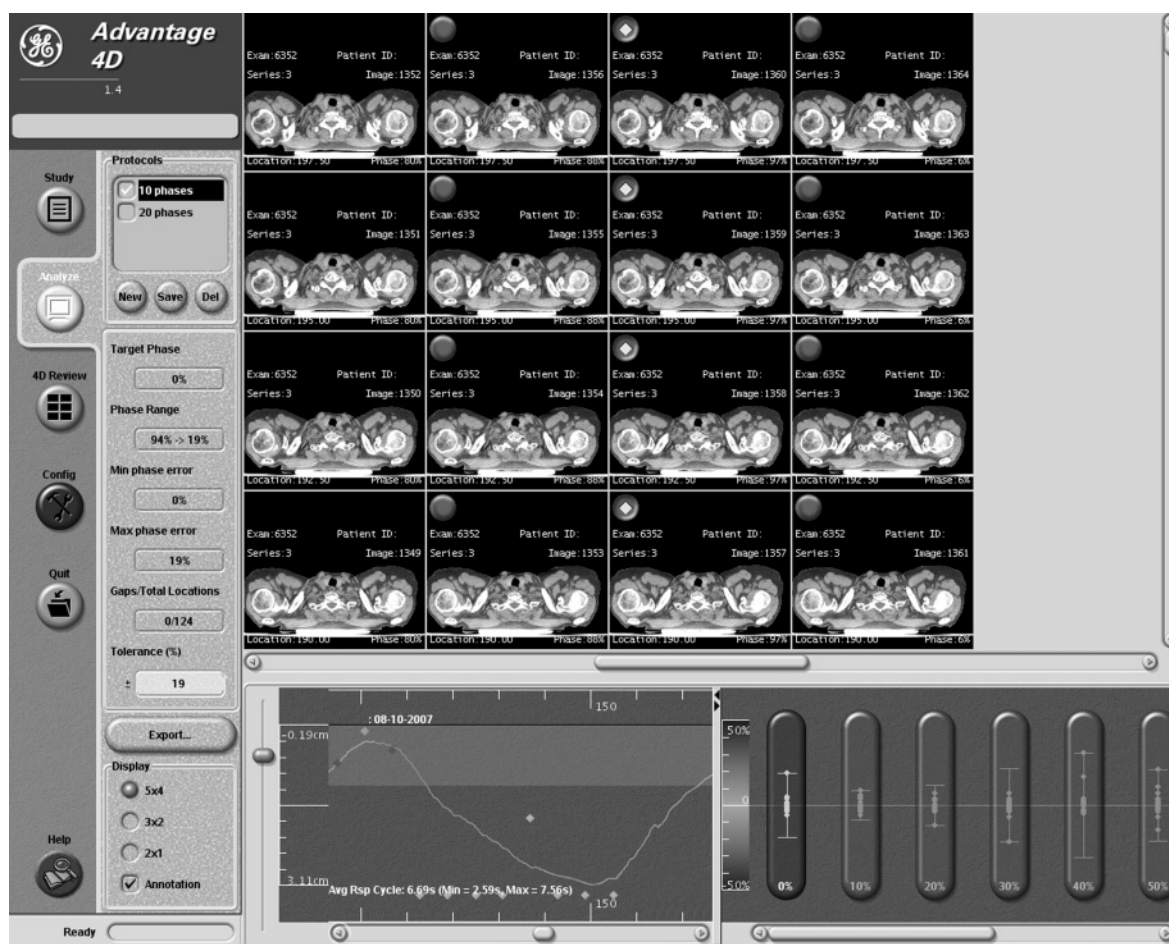
Figure 10.12 A 4D-CT study display from GE AdvantageSim MD. The respiratory cycle is represented by the waveform at the bottom of the screen; each column contains images acquired during the same part of the cycle. (Courtesy of GE Healthcare.)
