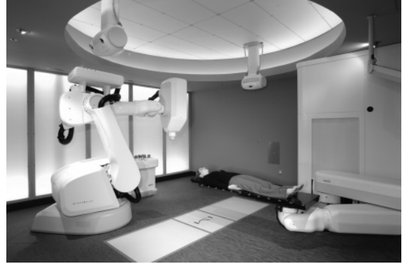
Figure 12.7 CyberKnife Robotic Stereotactic Radiotherapy System. (Courtesy of Accuray Inc.)
