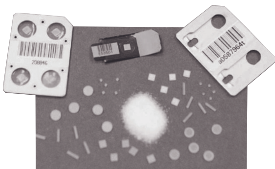
Figure 3.9 The variety of physical forms of thermoluminescent dosimeter (TLD) materials available. (Reproduced courtesy of Harshaw/Bicon NE Technology Ltd.)
