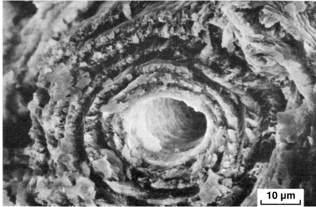
Figure 5.7. Scanning electron micrograph showing the mineral portion of osteon lamellae. The organic phase has been removed using ethylenediamine in a soxhlet apparatus. Reprinted with permission from [27]. Copyright © 1978, Academic Press.
